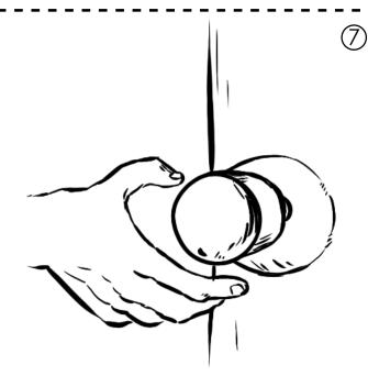
A wheel and axle is made up of a wheel with a rod attached to it. When the wheel is turned, it turns the axle with it.
