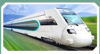
A type of train, called a Maglev train, uses magnets to lift it off the track so that it floats. Floating reduces
