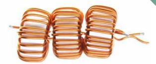
A coil of wire, wrapped around a piece of metal, becomes a magnet when electricity is run through the wire. This type of magnet is called an electromagnet. It can be turned on and off, by turning the electricity on and off.
