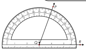
The protractor's arrow and pen hole is placed on the angle's vertex. The 0° line is placed over one side of the angle. Read the measure where the other leg of the angle intersects the protractor.
