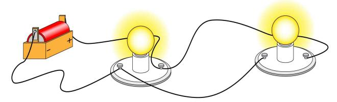
If a light bulb is missing or broken in a parallel circuit, will the other bulb light? Explain.
