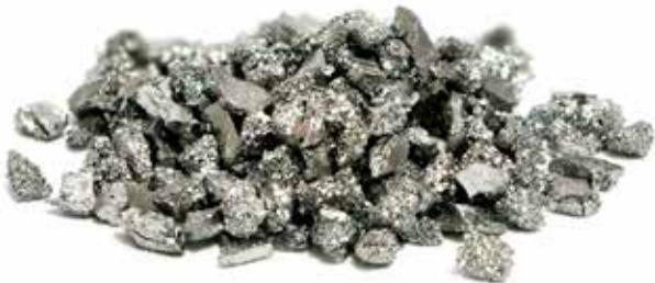
At normal pressure, tungsten has the highest melting and boiling
