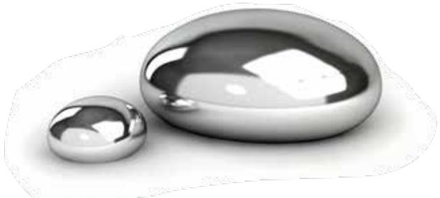
At room temperature (68–72 °F, 20–25 °C), mercury is the only liquid metal. Solid mercury melts at  $-37.89$  °F ( $-38.83$  °C).
