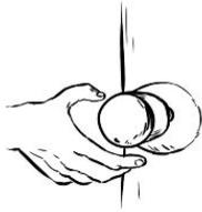
When you turn the large knob on a door, a rod on the inside releases a latch that holds the door closed. It would be difficult to turn the rod, if the knob wasn't attached to it.
