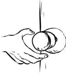
When you turn the large knob on a door, a rod on the inside releases a latch that holds the door closed. It would be difficult to turn the rod, if the knob wasn't attached to it.
