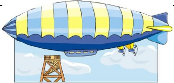
High above many big sporting events, you're likely to see a blimp sailing through the sky. Blimps are related to hot air balloons. The main difference is that blimps use the gas helium, and they can move in any direction. Hot air balloons are only able to move vertically, up and down. When a hot air balloon moves in any other direction, it's because the wind is blowing the balloon along.
